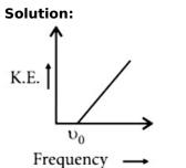
Frequency  $\rightarrow$ The maximum kinetic energy of photoelectron ejected is given by K.E. =  $hv - W = hv - hv_0$ where work function depends on the type of material. If the frequency of incident radiation is greater than  $v_0$  only then the ejection of photoelectrons start. After that as frequency increases kinetic energy also increases.
